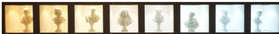
Figure 3: A representation of different correlated colour temperatures from warm white to cool white. The higher the Kelvin degrees, the cooler the colour appearance. (Photo: Emrah Baki Ulas)
